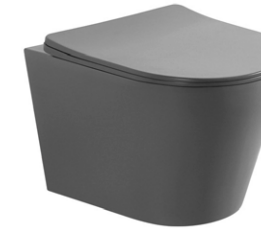
LX-1905TMG/1905MG Tornado/Rimless Washdown Flushing Wall-hung Toilet Vitreous China 525x360x320mm P-trap 180mm
