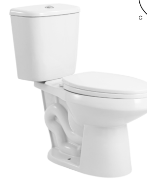
LX-2749A Siphonic Flushing Vitreous China 730x395x820mm S-trap 300mm
