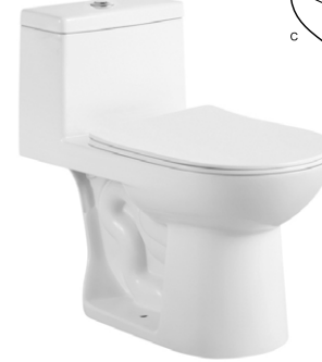
LX-2734/2734MW Siphonic Flushing Vitreous China 685x365x670mm S-trap 300mm
