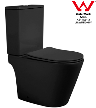
LX-2904TMB Tornado Washdown Flushing Two-piece Toilet Vitreous China 630x385x815mm P-trap 180mm
