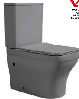
LX-2914TMG Tornado Washdown Flushing Two-piece Toilet Vitreous China 635x385x820mm P-trap 180mm
