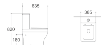
LX-2914TMB Tornado Washdown Flushing Two-piece Toilet Vitreous China 635x385x820mm P-trap 180mm
